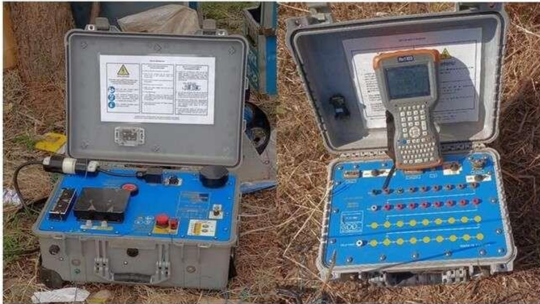
Figure 13: GDD IP Transmitter model TX4 and IP Receiver model GRx 8 –32
